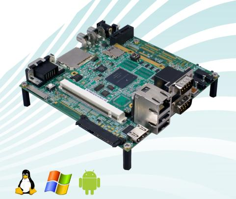
iW-RainboW-G7D is a generic Q7 Carrier board targeted for quick validation of high performance Q7 R1.20 compatible CPU modules. This board has rich set of features including Video IN/ OUT, Audio, Wired/ Wireless communication, PCIe, USB and various serial communication ports. Being a nano ITX form factor with120mmx120mm size, the board is highly packed with all necessary onboard connectors to validate complete Q7 supported features.
